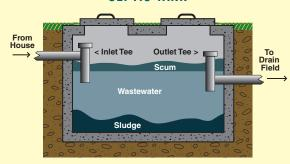
Incoming solid matter sinks. Soap and grease float. The tank has an outlet baffle to hold in undigested waste. Only clean water should leave the tank and enter the lateral pipes.
