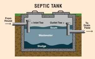
Incoming solid matter sinks. Soap and grease float. The tank has an outlet baffle to hold in undigested waste. Only clean water should leave the tank and enter the lateral pipes.
